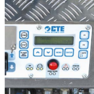
DIAGNOSTIC TOOL INTEGRATED IN THE CONTROL PANEL
